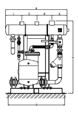
All connections are screwed gas female ISO 7/1 Rp except the pump connections which are flanged DIN PN 16. Screwed flanges can be supplied on request.
