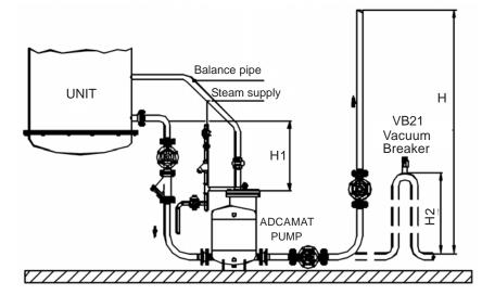
Drainage of a single unit under vacuum (max 0.2 bar abs).
