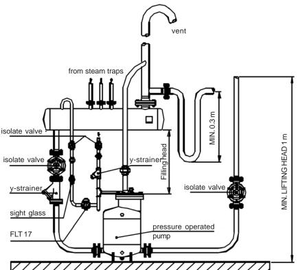
Condensate recovery - open system. The pump removes high temperature condensate without cavitation problems.
